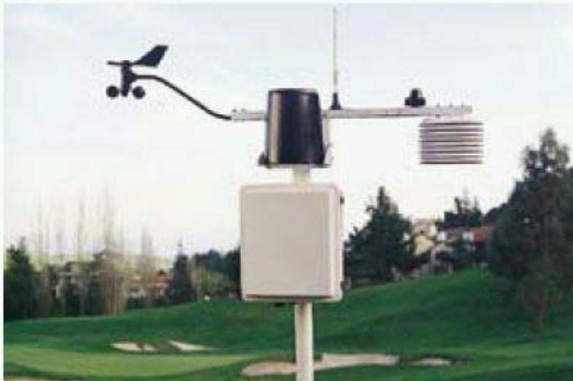
*Small weather stations are affordable and can communicate directly with irrigation controllers to adjust programs automatically in response to Evapotranspiration..*
